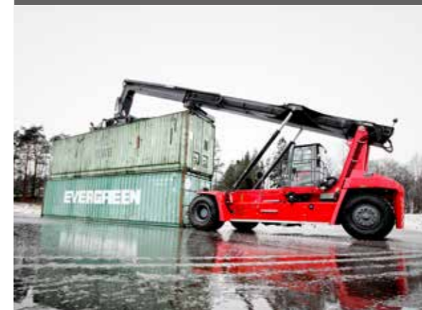
Precise lifting of long container end-on - 40 ft
