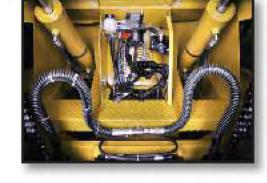
**ELECTRICAL PANEL:** Electrical system maintenance is easy through a hinged weather tight compartment located on the front of the unit between the forks.
